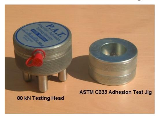
The PAT tensile testing jig is designed for pull off testing of thermally applied coatings in accordance with ASTM-C633 using the PAT adhesion tester.
